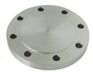
A Blind flange is round plate which has all of the relevant boltholes but no center hole, and because of this feature this flange is used to close off the ends of a piping systems.
